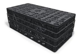
Dimensions:L 1200 x W 600 x D 420 mmGross Volume:302 LStorage Volume:290 LVoid ratio:96 %Materials:PolypropyleneRecyclable:100 %Approximate weight:11.5 Kg
